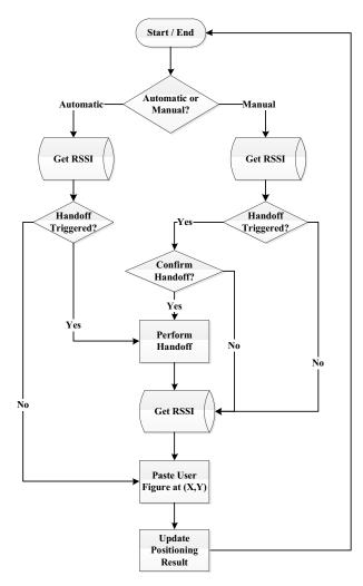
Figure 2. Flow chart for handling positioning handoff.
