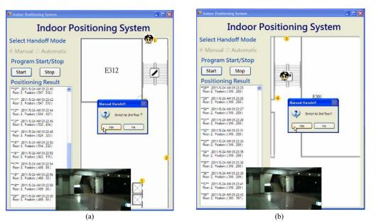
Figure 6. The prototype system prompted for confirmation of handoffs in manual mode. (a) going downstairs from the  $3^{rd}$  floor (b) going upstairs from the  $2^{nd}$  floor
