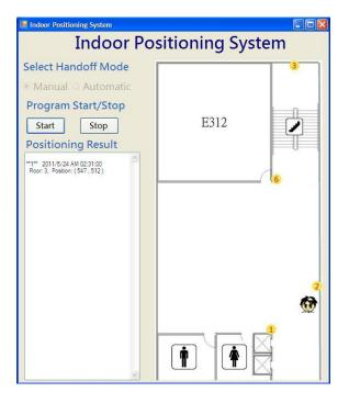
Figure 5. The graphical user interface of the prototype system with the manual handoff mode selected.
