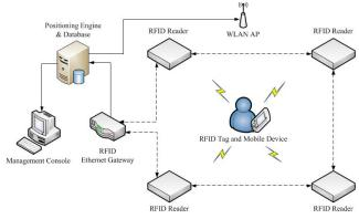
Figure 1. Schematic diagram of the proposed personal navigation system.
